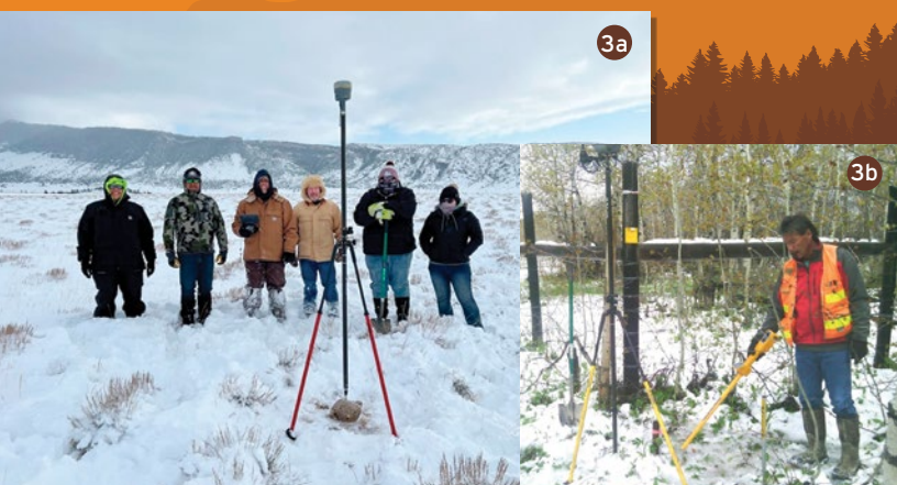
Figure 3a: Tribal surveyors search for PLSS corners with the Bureau of Indian Affairs land surveyor using the Real-Time Network in the Crow Coordinate System. Figure 3b: Rick Ollinger, a Blackfeet surveyor, searches for PLSS corners using the Blackfeet Coordinate System. Figure 4: The collaboration between tribal nations, the states of Montana and Wyoming, and several U.S. federal agencies, made it possible for anyone surveying, designing, or mapping GIS data to coordinate data into one base and access it anywhere.
